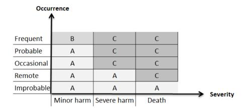
Source: Graphic freely adapted from: HASTENTEUFEL, Mark; RENAUD, Sina. Software als Medizinprodukt - Entwicklung und Zulassung von Software in der Medizintechnik. Springer Vieweg Wiesbaden. 2019. [75] (created with Microsoft® Excel 2010); Classes A, B, and C represent software with the lowest, medium and highest risk
